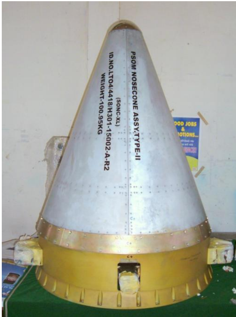
Manufactured Strap On Nose Cone (SONC) for Launch Vehicle
